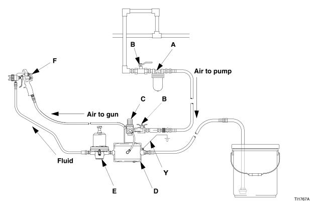
Fig. 4. Low pressure, non-circulating system, mechanical fluid regulator
